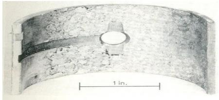
Fatigue of bearing lining. Fig. 1-10
