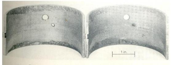
Fig. 1-12 Fatigue caused by an hourglass-shaped shaft.
