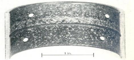
Fig. 1-8 Bearing with severe dirt embedment.
