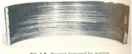
Fig. 1-9 Bearing damaged by scoring.
