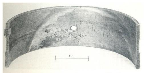
Fig. 1-11 Fatigue caused by a tapered shaft.
