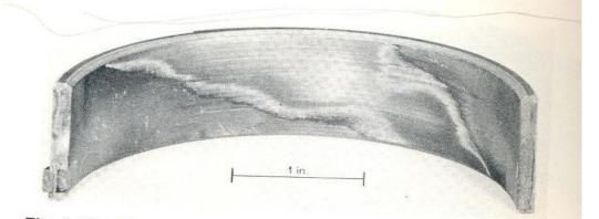
Fig. 1-15 Skewed-wear pattern caused by a bent connecting rod.
