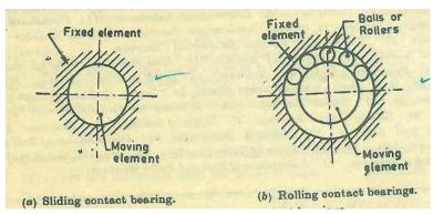
Figure. 2 Sliding and Rolling contact bearings.
