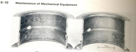
Fig. 1-13 Fatigue caused by a shifted bearing cap.
