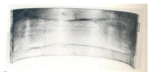
Fig. 1-14 Bearing worn in the center by a barrel-shaped shaft.
